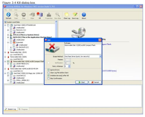
To choose an erase method, select one from the drop-down list. Erase methods are described in Chapter 5 Descriptions of Erase/Wipe Parameters in this guide.
