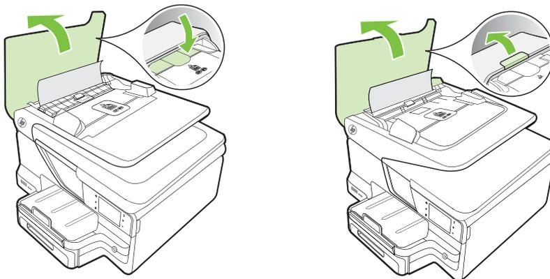
2. Lift the tab located on the front edge of the automatic document feeder.
